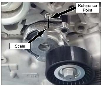
(23) Rotate Auto Tensioner pulley bolt to the right until it stops at the stopper. Mark another position where align with the reference point marked in (18).
