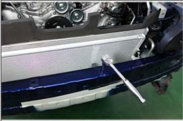
(5) Shave 2mm of the pipe clamp on the A/C condenser of the passenger's side as shown below.
