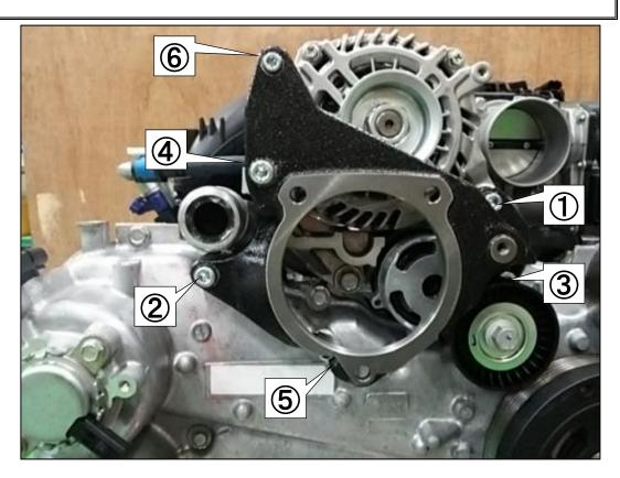
(7) Install the V-ribbed Belt temporarily installed in 3.(5) to \*7. Install the V-ribbed Belt to the engine.
