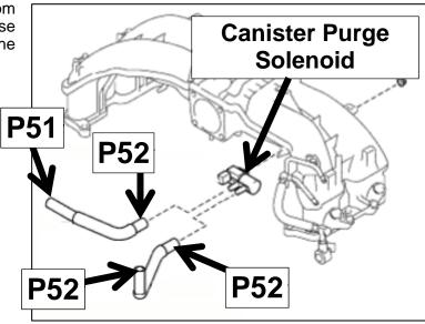
(40) Reinstall the canister purge solenoid. Place the throttle body and A/C compressor back in place.
