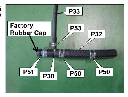
(11) Install the Hose 10mm to the intake manifold.
