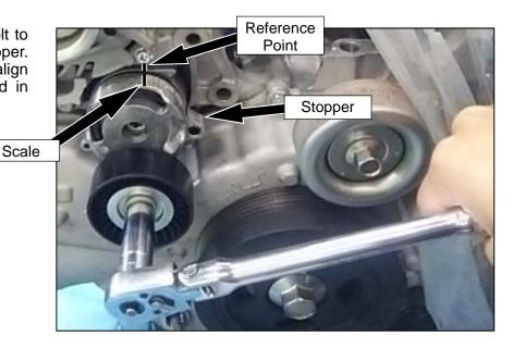
(24) Remove Auto Tensioner from the alternator bracket.
