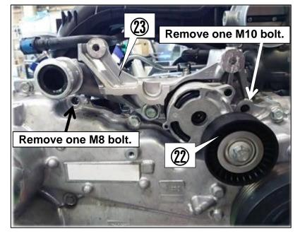
(18) Temporarily install @alternator removed in 1.(21) to @alternator bracket.
