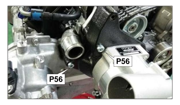
(6) Make sure the V-ribbed Belt is not caught in the Supercharger Bracket or engine. Tighten each cap bolt in several times in the order shown in the diagram below.
