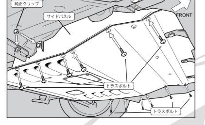
Notice \*When using the jack-up point, please remove the under panel body.
