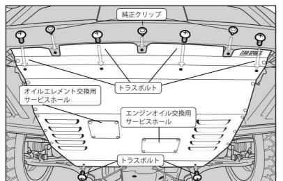
3. Referring to the illustration, temporarily fix the under panel to the front section using the original clip, the front bracket and rear stay that were installed earlier, and the truss bolt.
