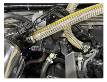
The hose band for the hose connected to the oil catch tank is included. use things
