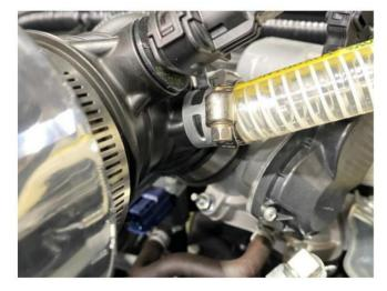
Insert the included 14ÿ joint pipe into the intake hose. Use the genuine hose clip as is.
