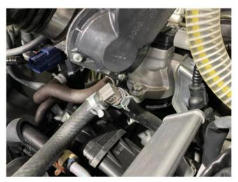
The catch tank body is installed behind the ABS on the left side of the vehicle. When you remove the blow-by pipe, the water pipe also comes off. Use one ABS fixing bolt. Then, connect the water hose with the included 8ÿ elbow pipe. The IN hose from the engine and the OUT hose go to the intake pipe.Use the genuine hose clip as is.
